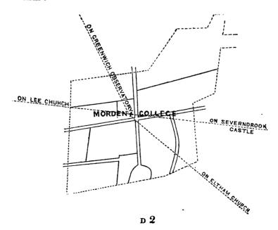
The main lines should be selected, as much as possible, with reference to permanent well-defined objects, such as churches, &c. In other cases it will be desirable that the extremities of the lines (or of some of them at least) should be marked, and preserved on the ground by stones or posts, or by trees, planted there so as to admit of the points being referred to at a future time.
